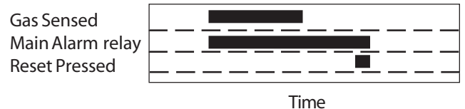
Main alarm switch in 'C' position
